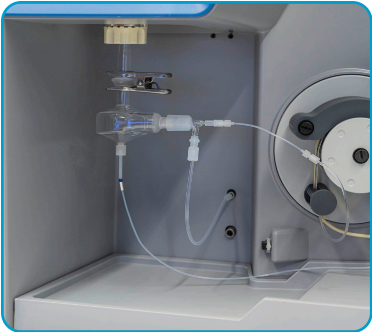
MEINHARD® OneTouch nebulizer includes pre-fitted fluoropolymer liquid and gas lines. Shown installed on iCAP PRO Series ICP-OES
